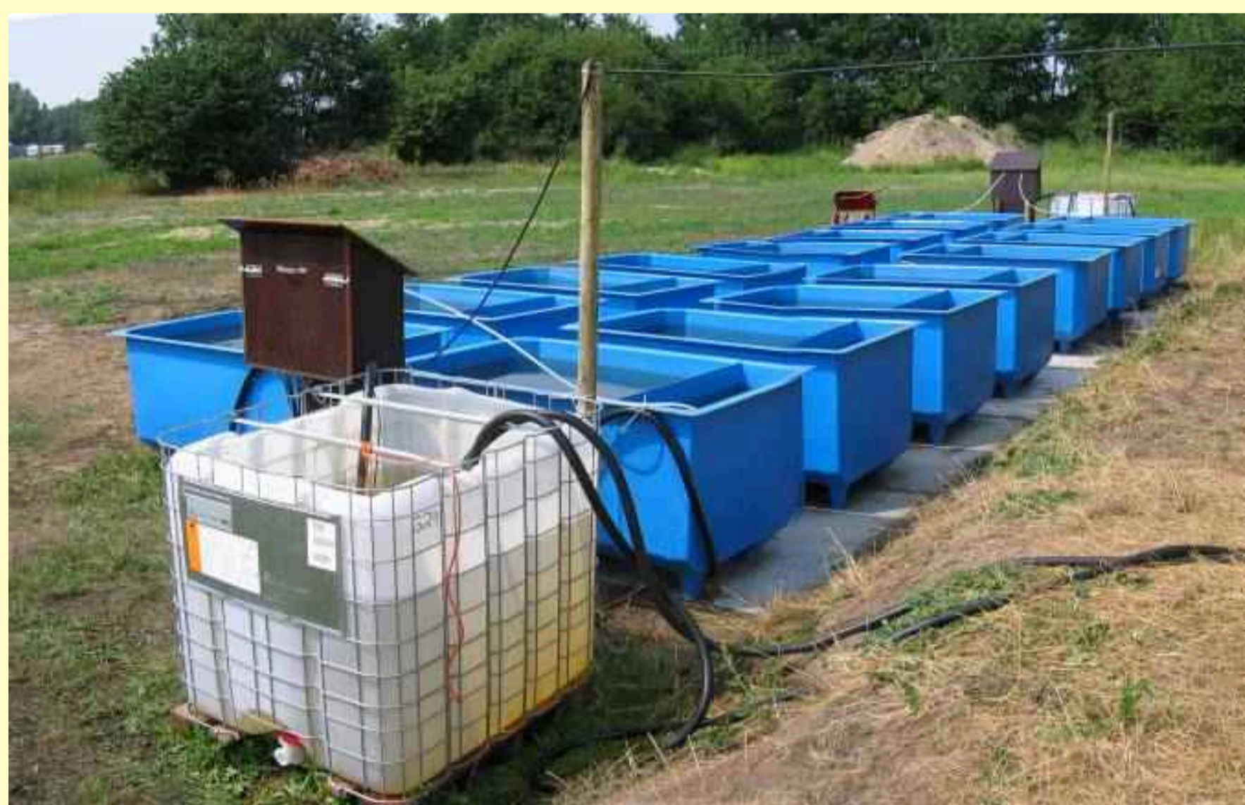
STP Horstermeer, The Netherlands Rather high loaded activated sludge process Ongoing research project Technical filtration Feed also filtered waste water Food web studies, harvesting of Daphnia
